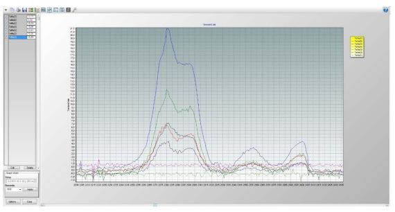
Figure 7. Test data from a pull of a 3 ton vehicle. The figure show data from 7 strain gauges.
